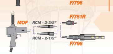
The diagram to the side summarises the full fitting equipment required for **Tuberal** tool driving.
